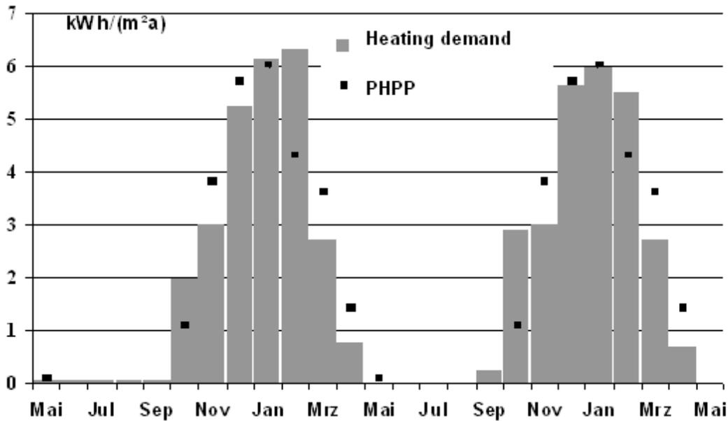
Figure 2: Heating demand for the renovated parts of the building, ground floor to second floor, for the first two time periods from May 2009 to April 2011; the 26 kWh/(m²a) calculated with PHPP was achieved despite two harsh winters.
