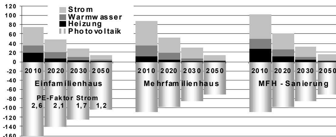
Figure 2: Optimization calculations in compliance with PPHP for a single-family home, a multi-family building, and a multi-family building renovation. Also depicted is possible yield from a photovoltaic roof array.
