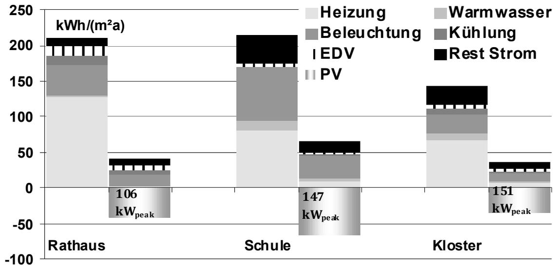
**Figure 3: Renovation of a non-residential building: primary energy balance of demand values for heating, hot water, cooling, lighting, IT, and residual current before and after renovation**
