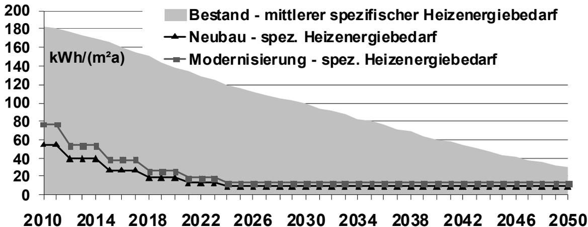
Figure 4: Specific heating energy demand for new buildings and modernization projects within the scenario and the resulting average heating energy demand for all buildings
