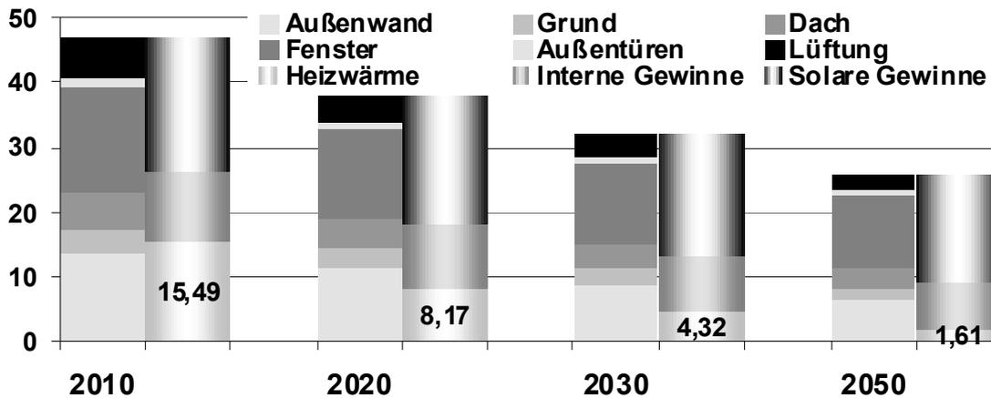
Figure 1: Passive house balance of components in Table 1 in a single-family home
